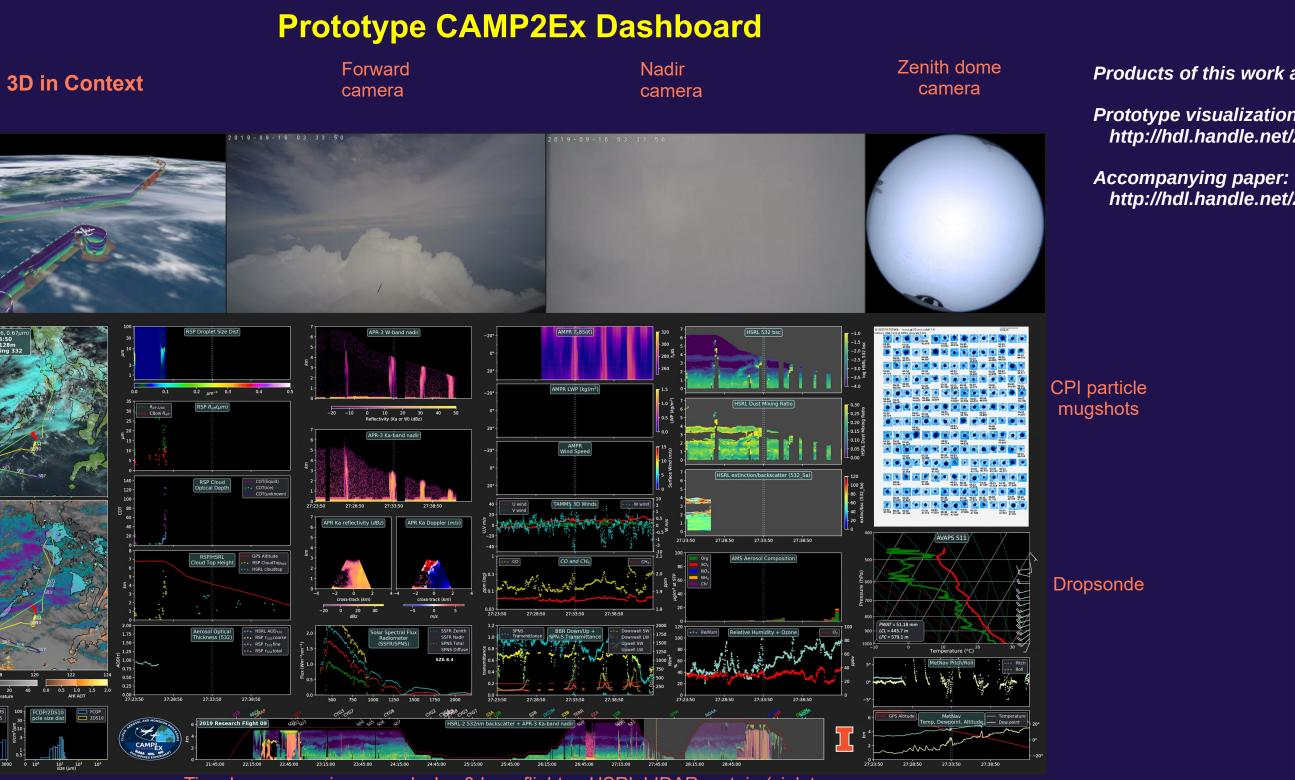
Time bar summarizes one day's ~8-hour flight. HSRL LIDAR curtain (violetgreen-yellow) shows aerosols beneath aircraft's track, interleaved with APR-3 precipitation radar (peach-purplish). Dashes mark limits of the time-window vis other plots.
