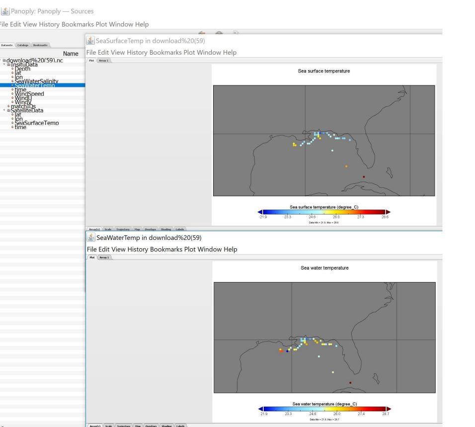
Since CDMS Group variables leverage existing CF standards, an off the shelf tool like Panoply that is CF-metadata aware can automatically interpret and map in situ and satellite group data independently just as if they were given in their separate CFcompliant source files.
